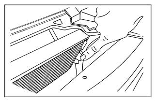
3. Remove the air filter from the housing by pressing the tab on the inboard side of the housing.
